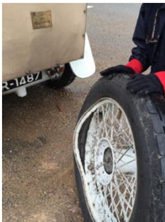
A shocking sight: split rim failure on 2154. Photo by Katie Forrest.
