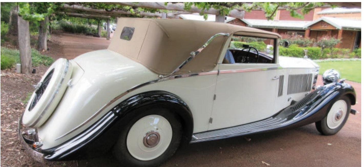
Charles and Diana Bush's 1936 25/30 chassis GWN36. This car had been imported from California in 2006, and Charles purchased it two years later. The original body was a Rippon limousine, rotten throughout. It was junked, and the car dismantled down to bare chassis with axles, springs engine and gearbox all removed. The chassis was restored, and a complete engine overhaul undertaken by Charles in his own shed. It then went to Roger Fry along with a picture of what Alan had in mind for the coachwork. Then to Matty Henderson for painting and Tony Parker for upholstery. This was a mammoth eight year restoration and is a credit to Charles and Diana.
