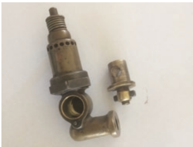
The starting carburettor that sits atop the inlet manifold is shown prior to being rebuilt.
