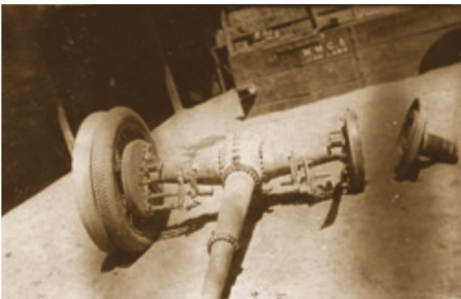
One of the box cars with a broken axle necessitating a repair back at camp.
