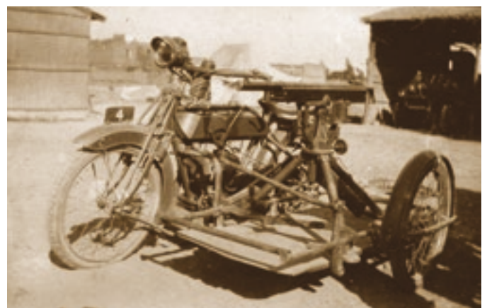
The New Hudson motorcycle initially used by the 1st Armoured Car Section and subsequently by the 1st Australian Light Car Patrol. It is fitted with a Lewis machine gun.
