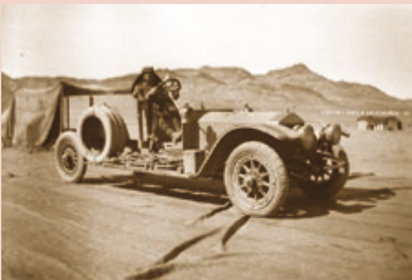
Chassis 60985 is shown following its requisition and removal of the original coachwork. Note the artillery wheels, whereas the later photograph shows the car has wire wheels, presumably fitted during its period of service. ( The Tank Museum , UK)
