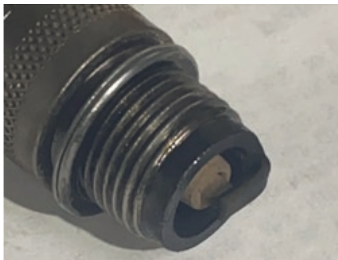
A spark plug after a twenty mile sprint to Swanpool following the successful renovations of the starting carburettor and the oil pressure relief valve.
