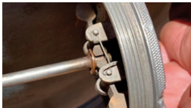
The float valve collar, a tortured soul. This collar controls the movement of the float valve and thus the amount of fuel coming into the chamber. At some stage this collar had been given a good larruping.
