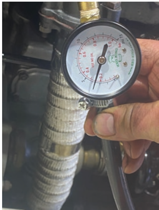
Testing after the oil pressure relief valve has been refitted to the engine. As per Rolls-Royce specification the oil pressure to the overhead gear is now 3 ½ psi.
