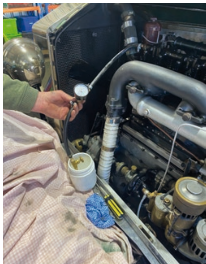
The rig made up to test the oil pressure to the overhead gear. By the time this measurement was being taken we were not surprised to see that oil pressure shown was vastly more than it should have been.
