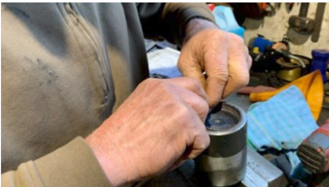
Removing the cup from the mould.
