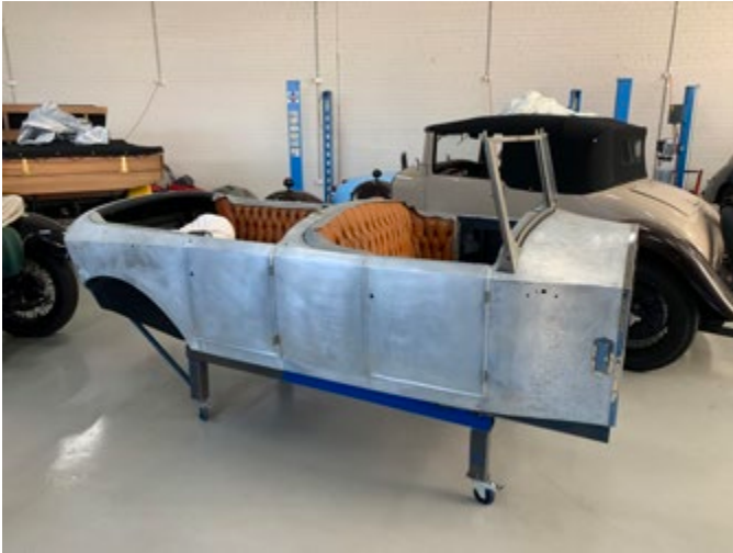
The body is aluminium over timber frame and appears to be constructed to a very high standard.
