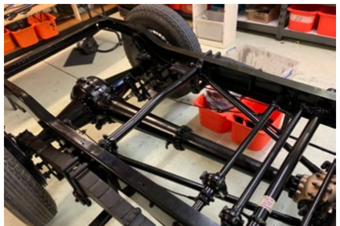
Rear of chassis showing the heavy differential.
