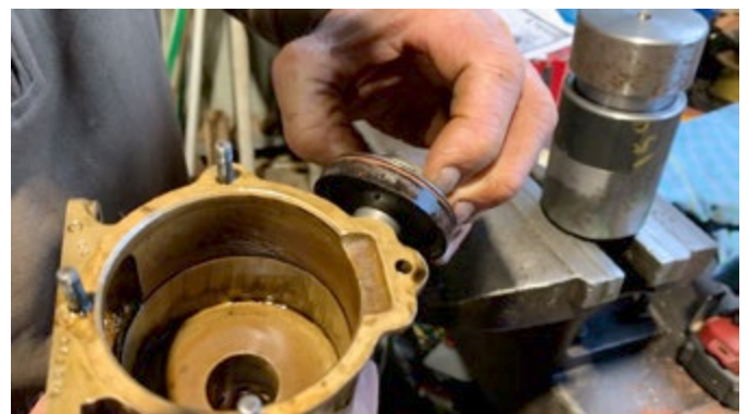
Chamber of the oil servo showing the 1/16th lip.
