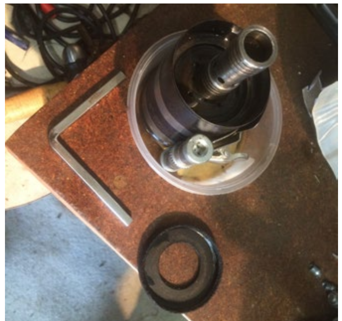
Compressing the leather washer.
