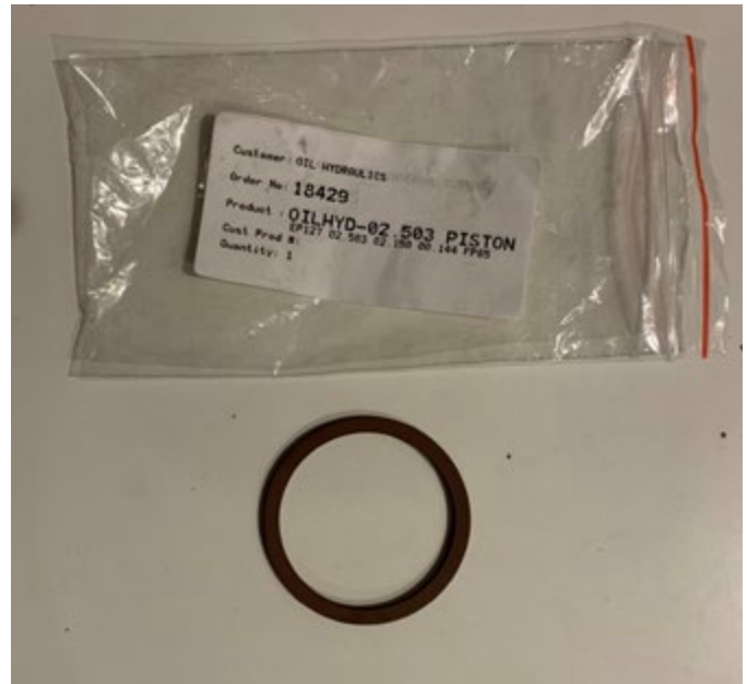
'O' Ring intended to replace the leather cup.
