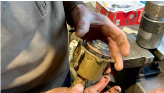
Leather cup clears the entrance to the chamber.
