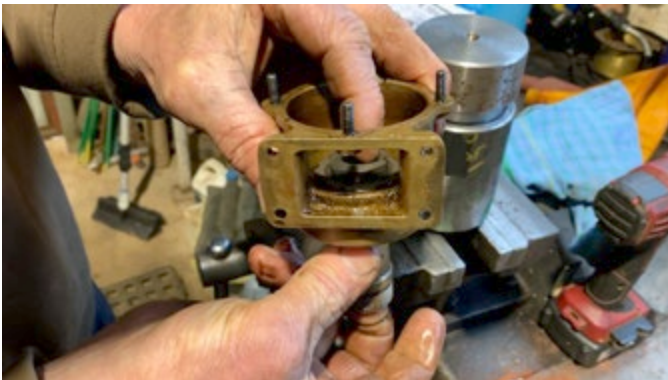
Leather cup in place in the chamber.
