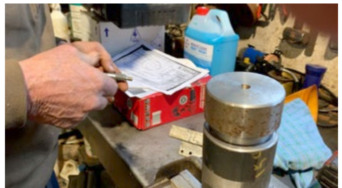
Mould for the leather cup.
