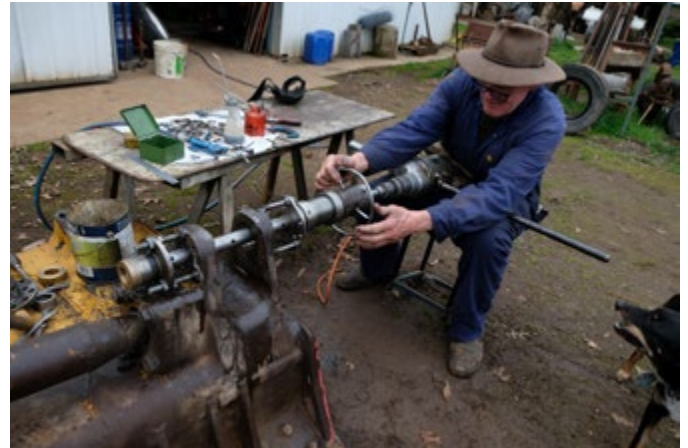
Bill Forrest line boring the bushes for the blade on a large bulldozer.
