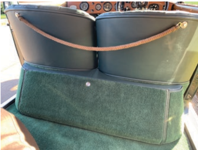
The car is fitted with a rear seat footrest in which a selection of tools are stored.
