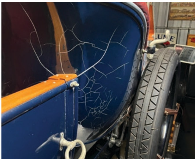
While the car as acquired was in good condition, however the paint had failed with severe cracking evident.
