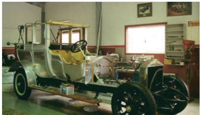
The coachwork for 2145 under construction.
