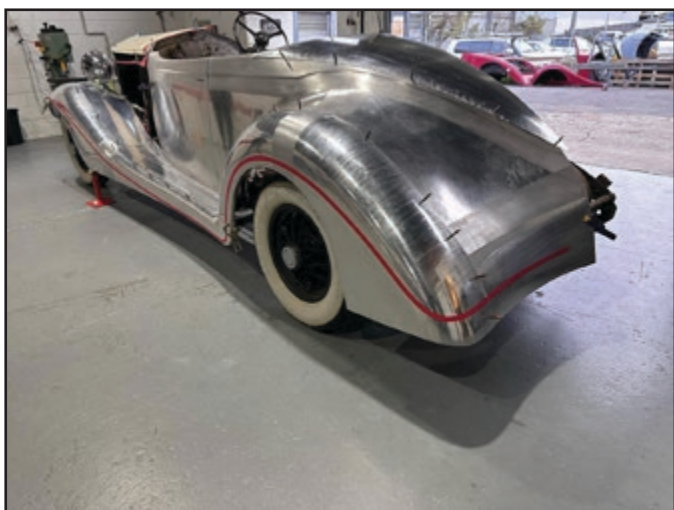
The rear boat tail of the new body. The offside is being completed, and then the onside will be duplicated by computer scanning. Note the remains of the third body outside the workshop.
