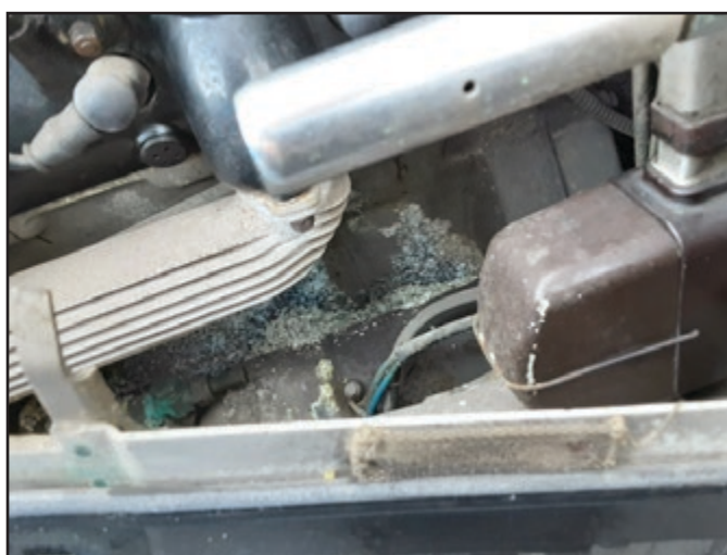
Significant corrosion was evident under the bonnet.
