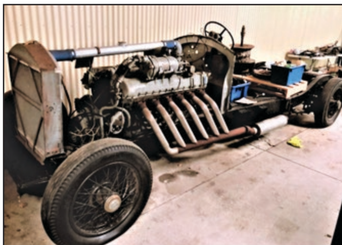
3AZ102, a shortened chassis fitted with a Rolls-Royce Merlin engine in South Australia (internet photo).
