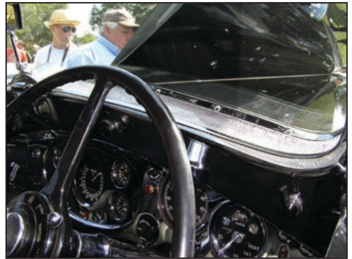
3AZ210 again, this time showing the ingenious insect screen that winds out with the lower edge of the windscreen in those hot French Riviera summers. Note also the ebonised dash treatment (Stuckey photo).
