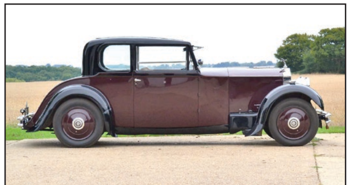
Bob Roberts recently purchased the very early 20/25, chassis GTR5, a 1930 coupe with very unusual body by Park Ward. The car features helmet wings along with a delightful mechanism such that when opening the doors, the running boards fold out allowing easy access.
