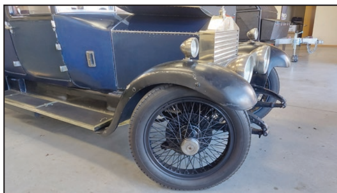
23 inch split rims fitted, May 31st, 2023.
