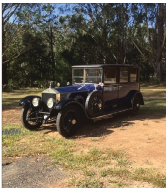
The Silver Ghost chassis 48RM of Ossie Millar. The wheelbase was extended prior to World War Two when the chassis was used as a hearse, while the current body dates from the 1970s or 1980s and was built by George Williams.
