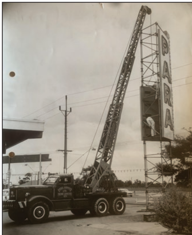
A Diamond T 980 Tank Transporter converted into a crane for the family business and at times tow-started by the Phantom I.
