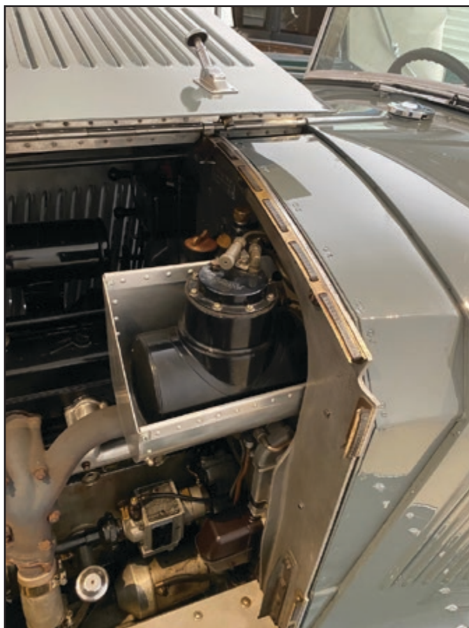
The heat shield fitted to overcome vapour lock.
