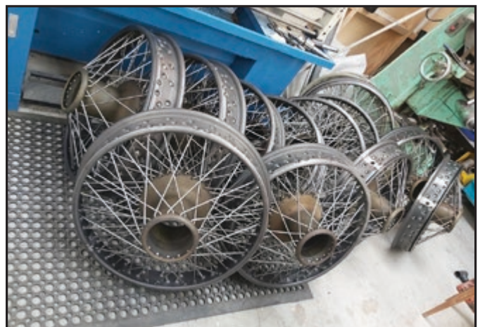
A new batch of Silver Ghost wheels produced by Vintage Rims in New Zealand just prior to the owner's retirement.
