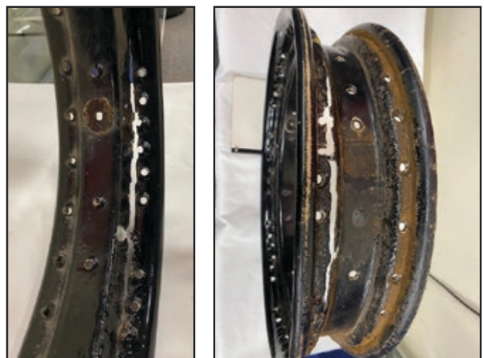
The damaged rim with the large split very evident. Surely a good case can be made for upgrading to new rims when restoring these cars.
