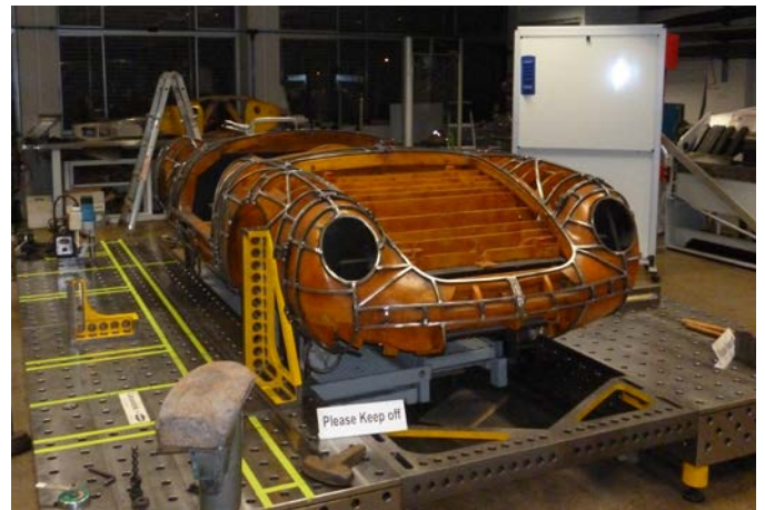
A timber buck used for panel forming and fitting.
