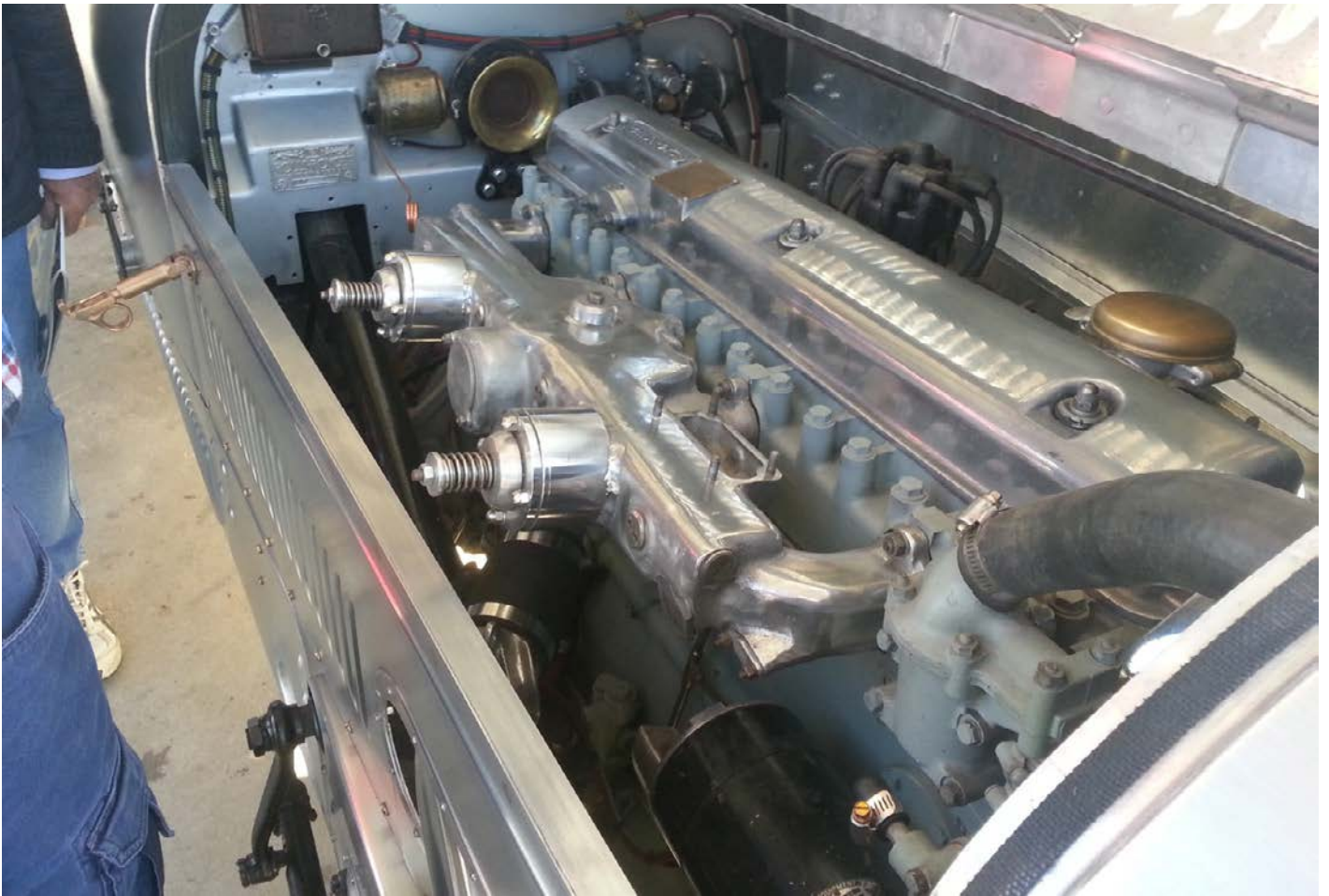
It's a brute - the straight eight military use Rolls-Royce engine. The car is fitted with a custom made supercharger and inlet manifolds.
