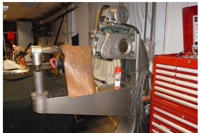
The panel hammering machine.
