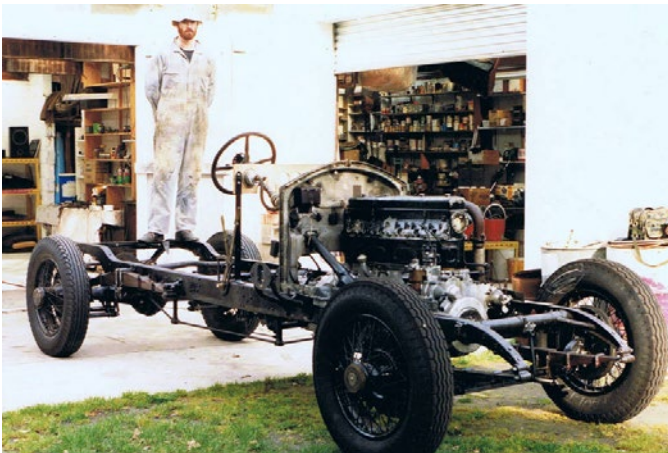
Coachwork removed, chassis dismantling to follow.
