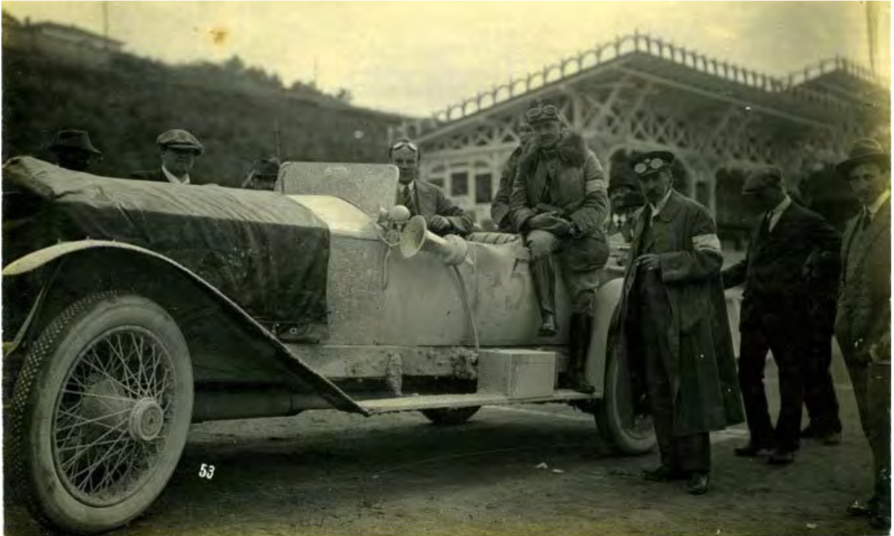
"Mr. Radley had a tight-fitting nightcap for his R-R of leather lined with asbestos and the engine started next morning with a quarter turn." Freestone from the Autocar.
