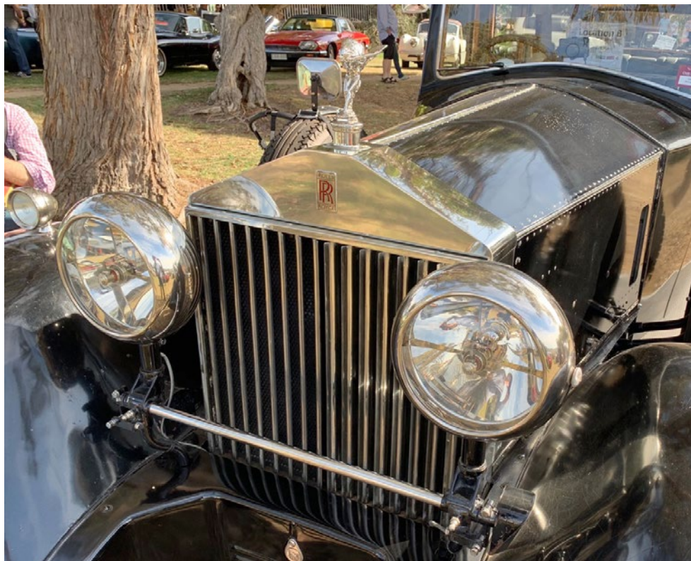
John Reis' Phantom displays the interesting headlamps made by Stephen Grebel of Paris, and typically offered to high end coach-builders.
