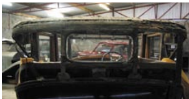
obvious distress to the roof covering opening-up roof reveals .....
