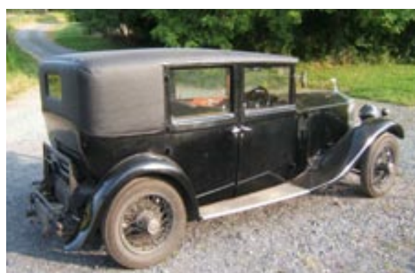
2010 - car re-assembled with new ash main frame, reusing as much of original as possible, & new leather-cloth roof covering
