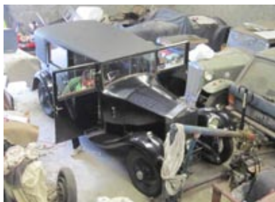
2010 - car re-assembled with new ash main frame, reusing as much of original as possible, & new leather-cloth roof covering
