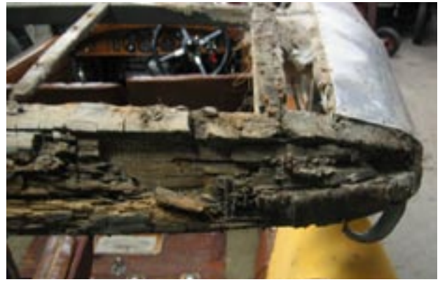
..... including extensive wet and dry rot!
