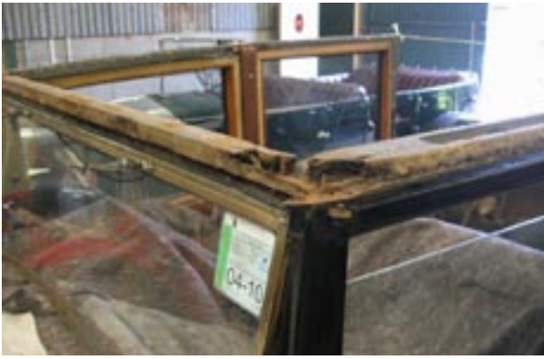
..... including extensive wet and dry rot!
