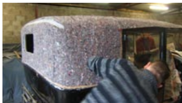
flock being fixed
