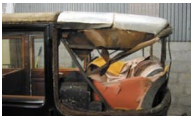
.....severe decay covered by tin sheets, cardboard, padding, & whatever you're having yourself .....
