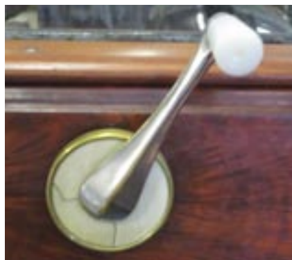
ply discs turned round, revealing original bone; new white resin knobs
