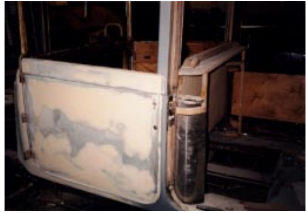
Original panels repaired and primed
