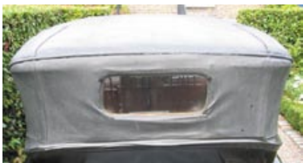
obvious distress to the roof covering opening-up roof reveals .....
