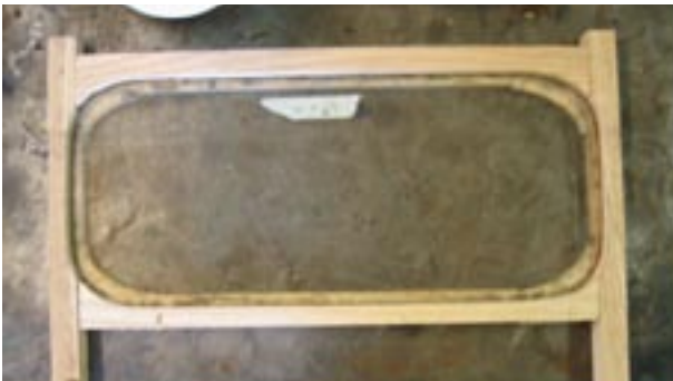
new ash frame for original glass of rear window
