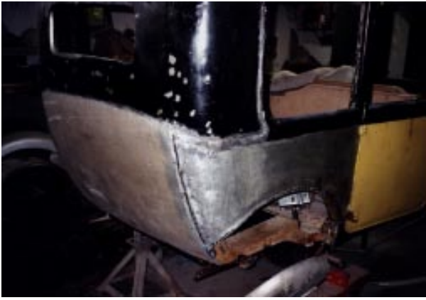
Original panels repaired and primed
