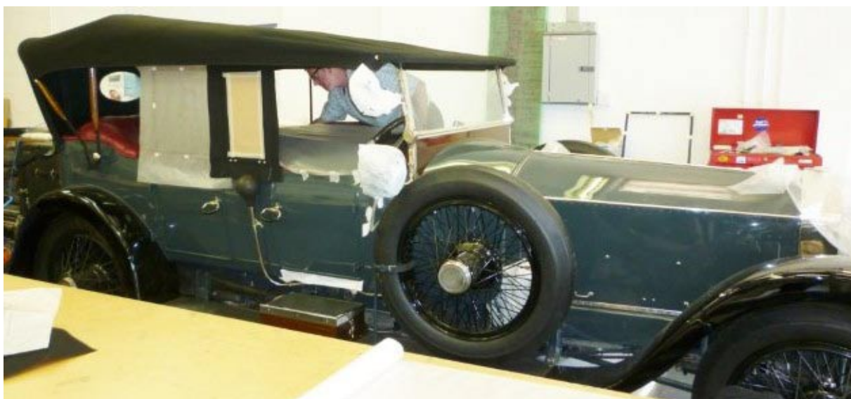
The new hood being made at the trimmer's
