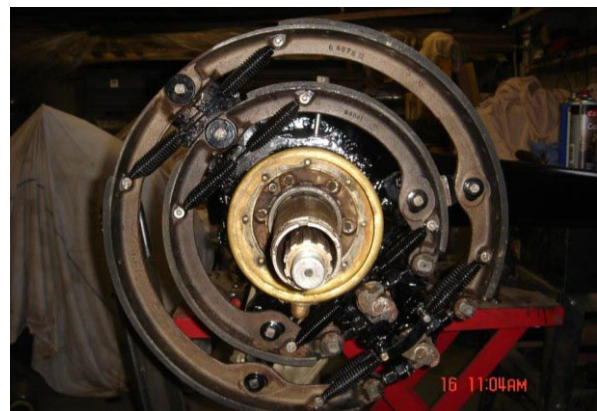
Brakes restored with new springs, etc
