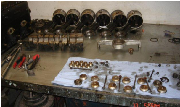
New pistons and rods etc: white metallurgy re-done
