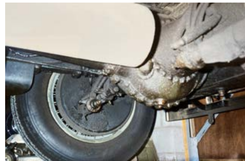
Left: The rear axle area 'as found' and indicates the depth and extent of the filth picked up by a chassis which has been regularly oiled but not cleaned.
