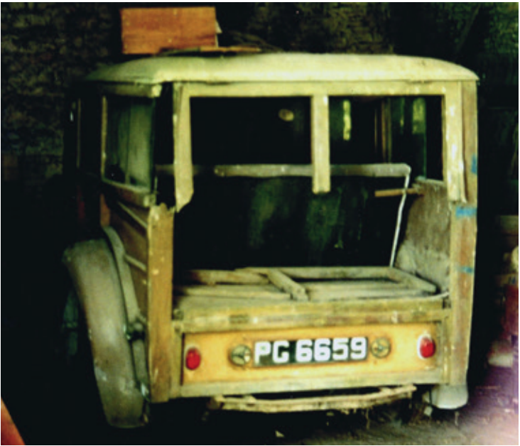
1998, the rear end damage is clearly visible with the main LH corner post completely removed above the waistline and the top tail gate broken up and the bottom tail gate in pieces in the back.
