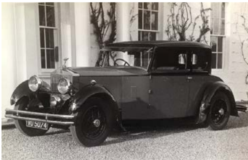
GTR5 after conversion to a fixed head (Photo credit: John Fasal)
