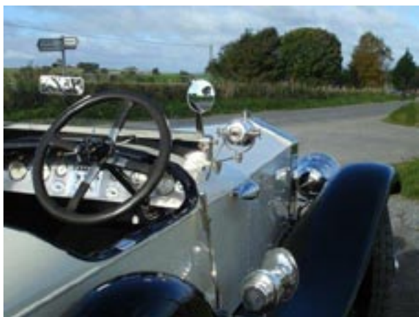
Details of the instrument panel and some of the silver plated fittings after restoration
