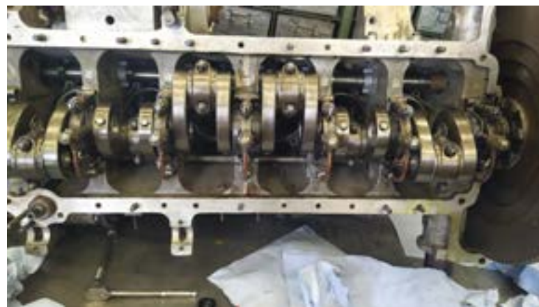
All conrods secured onto the journals. Notice the small socket drive we used, to avoid overtightening the bearings
