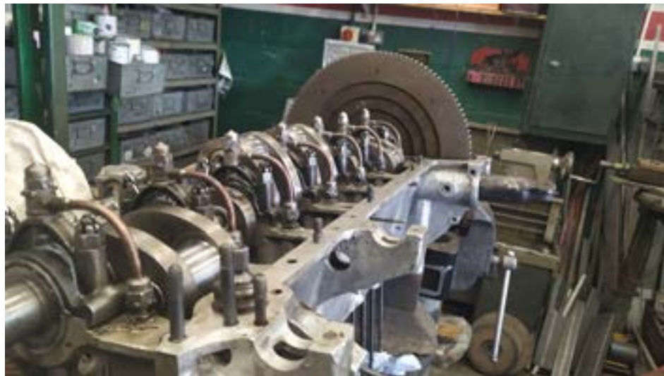
Main bearing oil delivery pipes fitted, with the main bearing caps tightened down.
