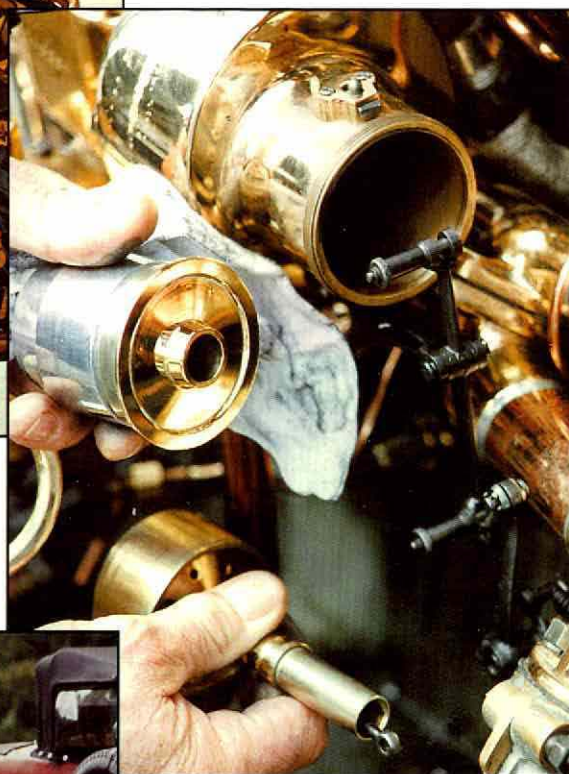
Barrie Gillings at work - changing the frictional properties of Malcolm Johns' carburettor from 22NK
