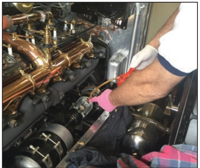
Most magnetos have an oiler provision under an oiler flap. Do not over-oil - a few drops at most. Some magnetos do not have provision for this oiler.
