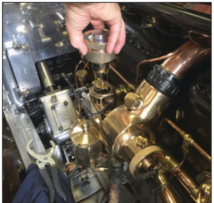
Care needs to be taken when removing and reinstalling the Air-valve on the carburettor when cleaning to ensure the needle is not damaged.
