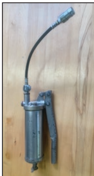
This old-style Tecalemit grease gun has a very handy refill cap at the top and a positive plunger lock. It holds about 500ml of oil which is plenty for mid-tour service (sphere, carbon shaft, torque tube - and maybe the kingpins).
