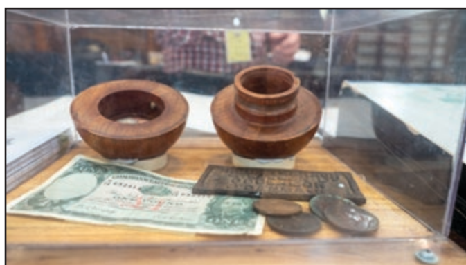
The store has a working Lampson Cash Railway System which uses a cash ball and gravity to send and return money to the cashier.
