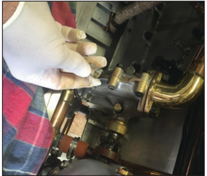
Penrite water pump grease should be used for the water pump.
