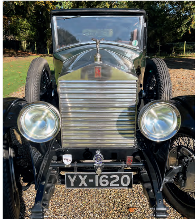
Being a 1928 20HP GBM37 has front wheel brakes but retains lovely horizontal radiator slats.
