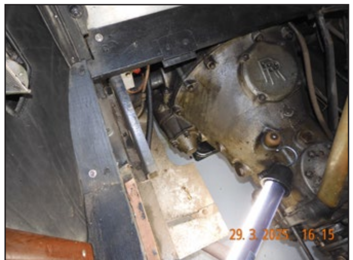
Removal of the starter motor starts by removal of the front floorboards.
