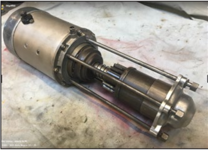
A file photo of an original starter from a small horsepower Rolls-Royce of the 1920s through the 1930s.
