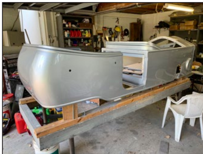
The newly painted body ready to be refitted to the chassis.
