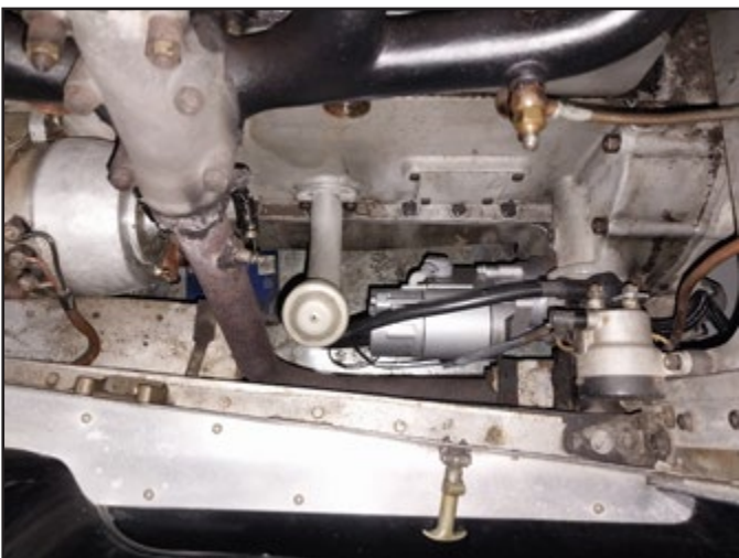
The new starter motor successfully fitted.
