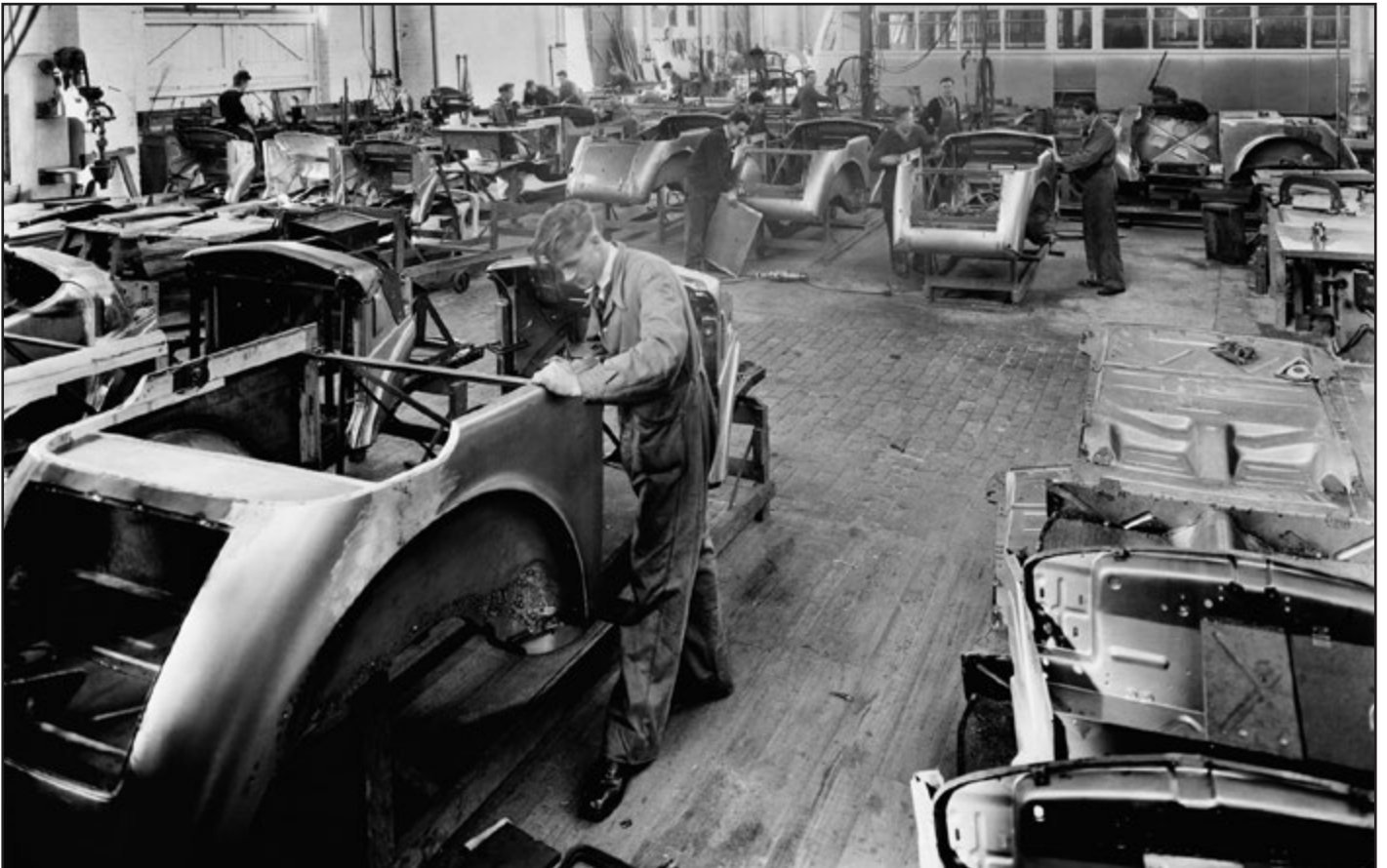
Anglia tourer bodies under construction at Malvern. Note also the railcar under construction in the background. (Photo: SLV)
