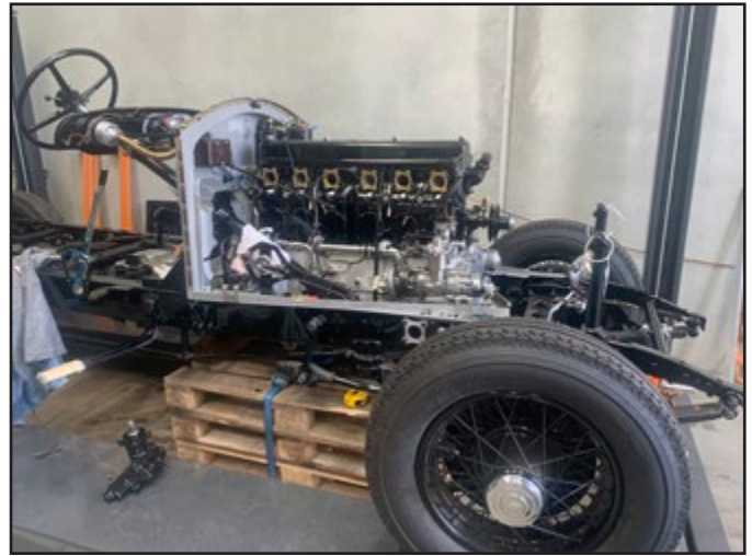
The engine is now all fresh following a complete rebuild.
