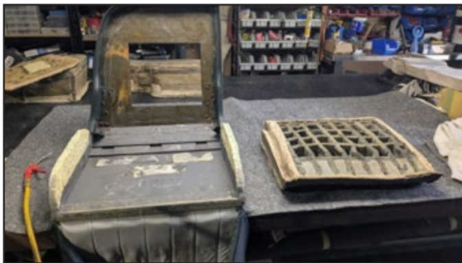
The passenger seat stripped down with the original Dunlopillo filling. The opening is for the toolbox under.
