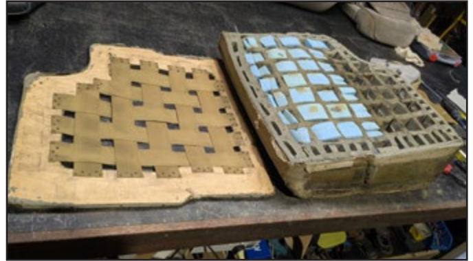
What was in the driver's seat. Someone had spent time putting new foam blocks into the old Dunlopillo.
