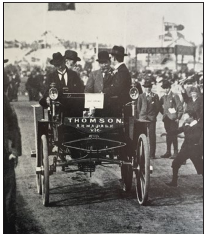
The Thomson steam phaeton pictured at a demonstration run in Bathurst in April 1900. The car was driven from Bathurst to Melbourne in 56 hours and 36 minutes to prove its viability. (Photo: VCCA Vic)
