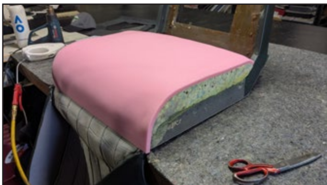
Squab ready for the leather to be replaced.
