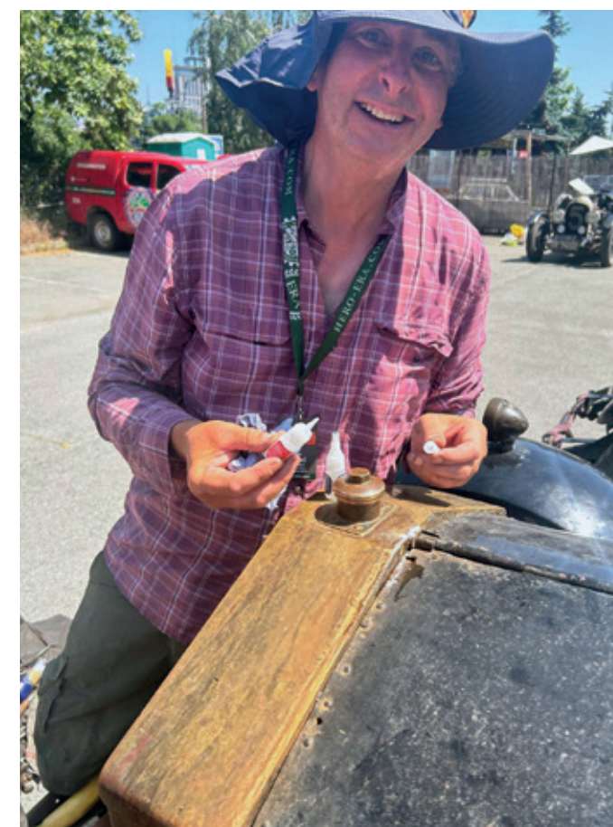
Co-driver, Nigel Parsons, applies Superglue to the top of the radiator to stop a minor leak.
