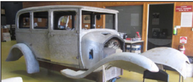
This all-aluminium body had been professionally built by Queensland Motor Bodies and was complete with its hardware and mudguards, but Frank was beginning to question whether it was what he really wanted.
