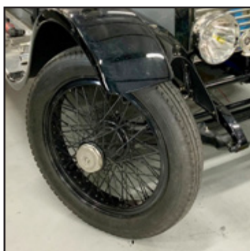
The 23-inch wheel fitted with 32 x 4.5-inch tyre on an early Twenty.
