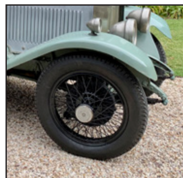
The later Silver Ghosts and early Phantoms used a wider 23-inch rim fitted with 33 by 5-inch tyres.
