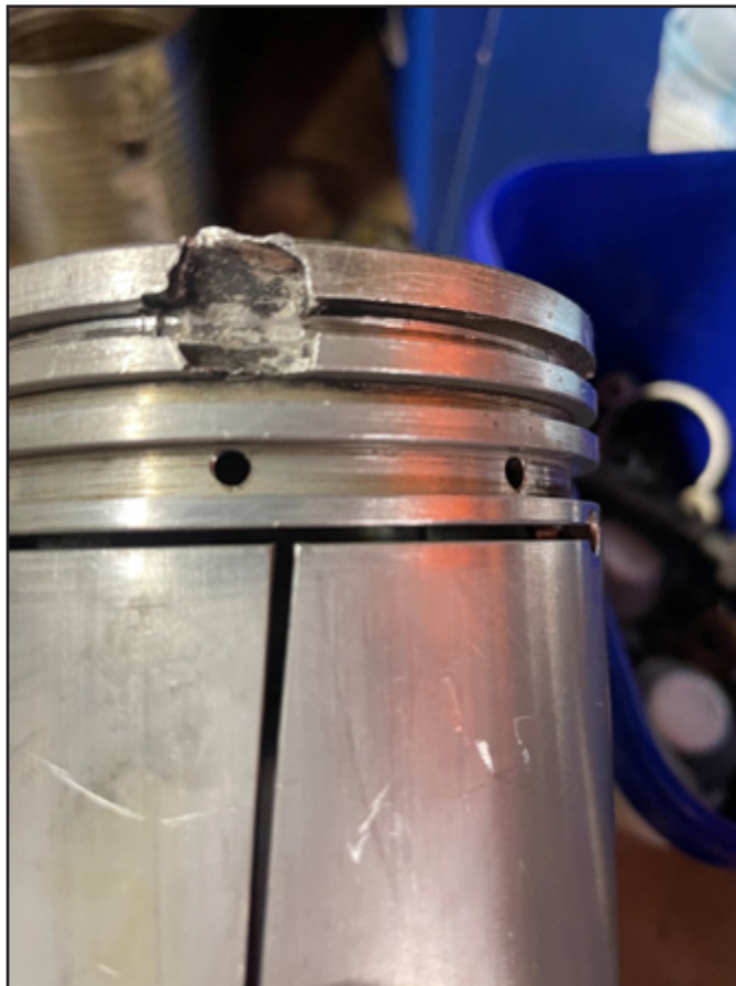
Some of the piston heads demonstrated almost catastrophic damage.
