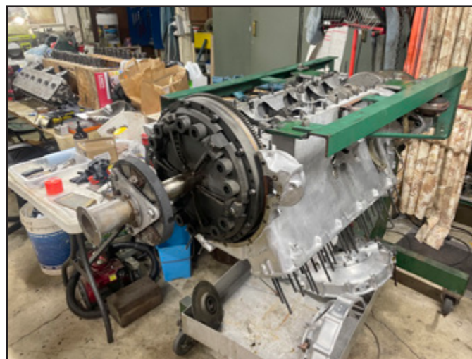
The engine cradle was perfect for the rebuilding.
